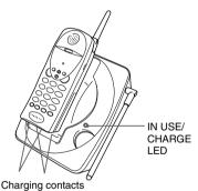
(5) Place the handset on the base unit. Be sure the IN USE/CHARGE LED lights. If the IN USE/CHARGE LED does not light, make sure the AC adaptor is plugged in securely and that the electrical outlet is working and not controlled by a light switch.
